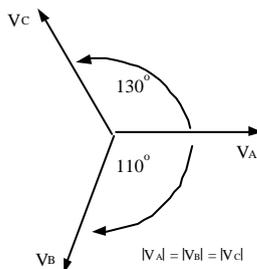
Fig. 8: A typical non-ideal source with balanced magnitude voltage
