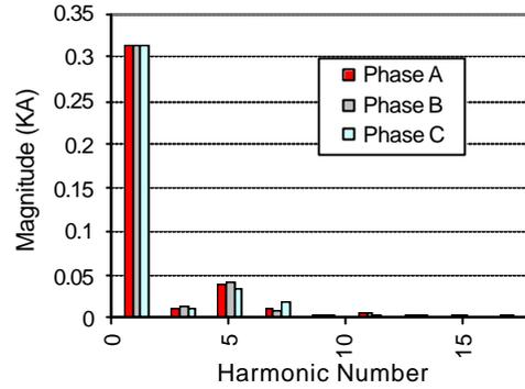
Fig. 9: Harmonic currents of the three-phase load under a non-ideal balanced voltage system
