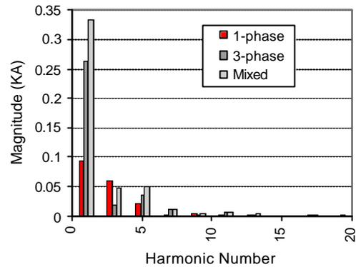
Fig. 16: The current harmonics under a non-ideal unbalanced voltage system
