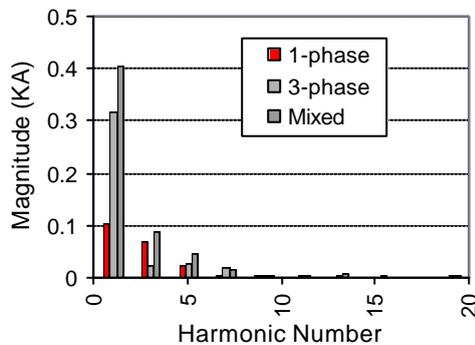
Fig. 15: The current harmonics under the non-ideal balanced magnitude voltage source
