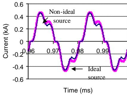
Fig. 14: The mixed current from ideal and non-ideal balanced voltage sources
