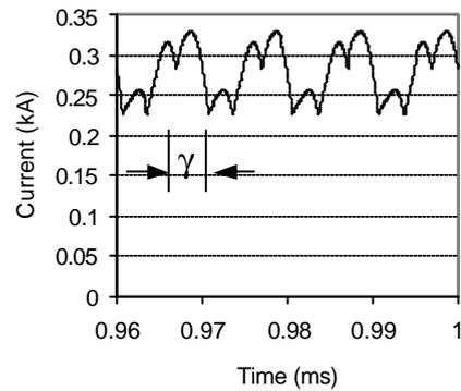
Fig. 13: The DC current when the rectifier is supplied by the non-ideal source
