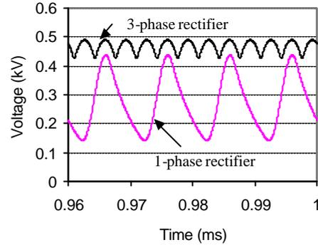
Fig. 3: DC voltage waveform
