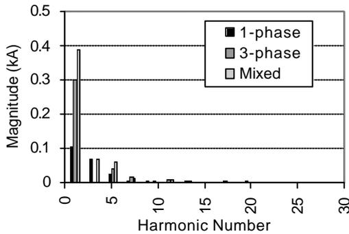
Fig. 12: Harmonic currents under a normal voltage system
