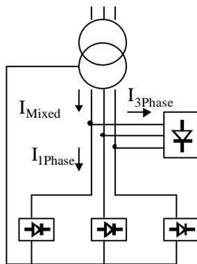
Fig. 2: Single-phase and three-phase rectifiers in a typical distribution system
