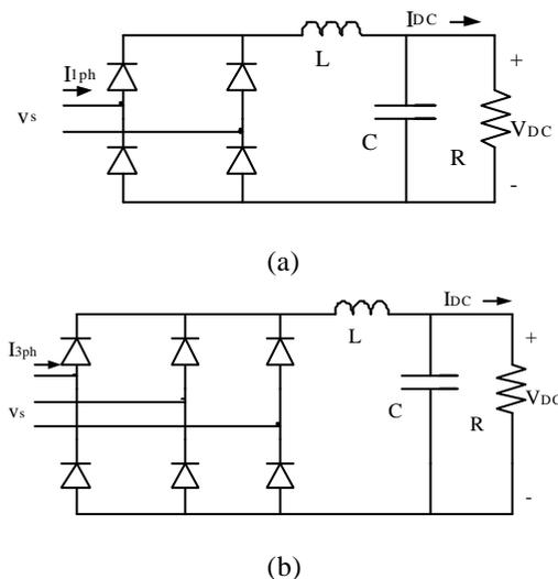
Fig. 1: (a) Single-phase and (b) three-phase rectifier
