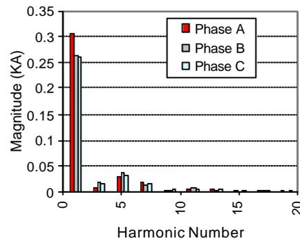
Fig. 10: Harmonic currents of the three-phase load under non-ideal unbalanced voltage system
