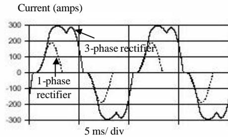
Fig. 4: Current waveforms of single-phase and three-phase rectifiers
