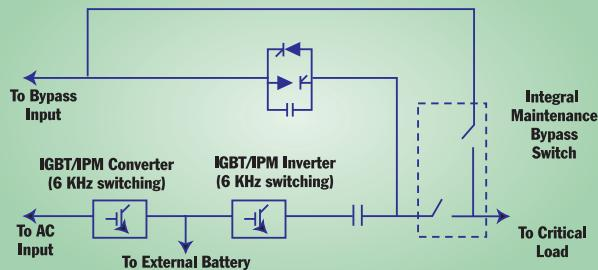
TOP: An on-line double-conversion system configuration for an IGBT/IPM, including a transistorized converter and inverter.
