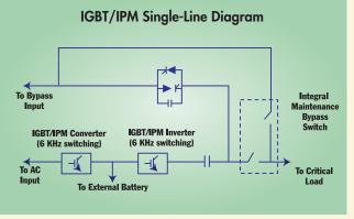
TOP: An on-line doubleconversion system configuration for an IGBT/IPM, including a transistorized converter and inverter.
